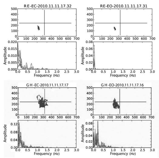
Figure 1. Sway and frequency analysis for (above) a stable person (above), and an unstable person (below); EC = Eyes Closed; EO=Eyes Opened
