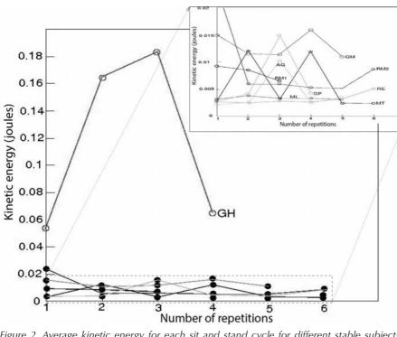
Figure 2. Average kinetic energy for each sit and stand cycle for different stable subjects (lower part of the figure, enlarged at upper right), and one unstable person, GH
